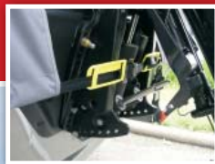
Stern Protector Pads guard against possible chaffing from connector straps
